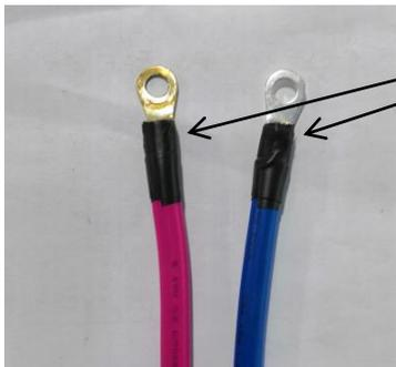
Width of insulating tape----- $12\text{mm} \pm 2$
