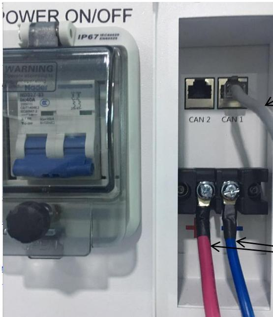
Take out of communication cable from accessory box, and Plug the communication cable
