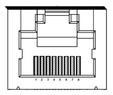
Figure 2.4 CAN interface definition
