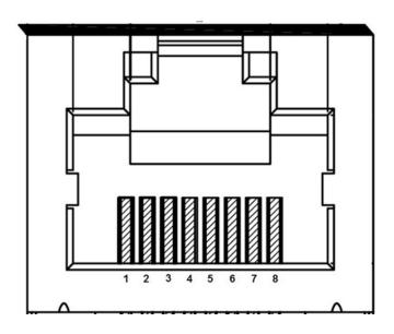
Figure 2.4 CAN interface definition
