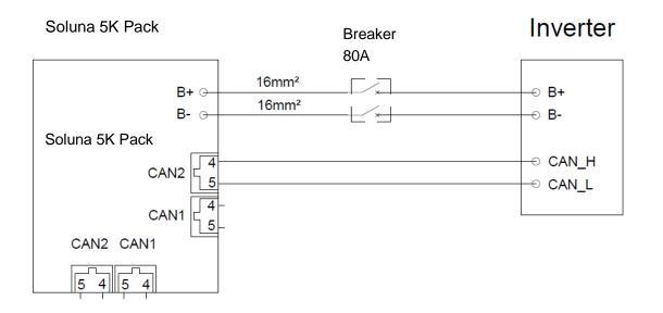
5.2 Multiple units are connected to the inverter, Please find the following diagram for details.
