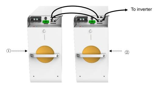
Figure 3.4 CAN communication wiring
