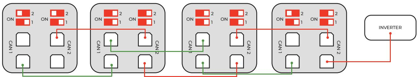
Please follow the diagram to adjust the switches, ensuring proper configuration
